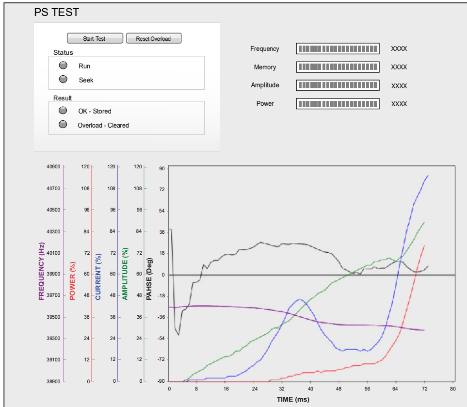
Figure A.11 Weld Graph, Defective Converter
