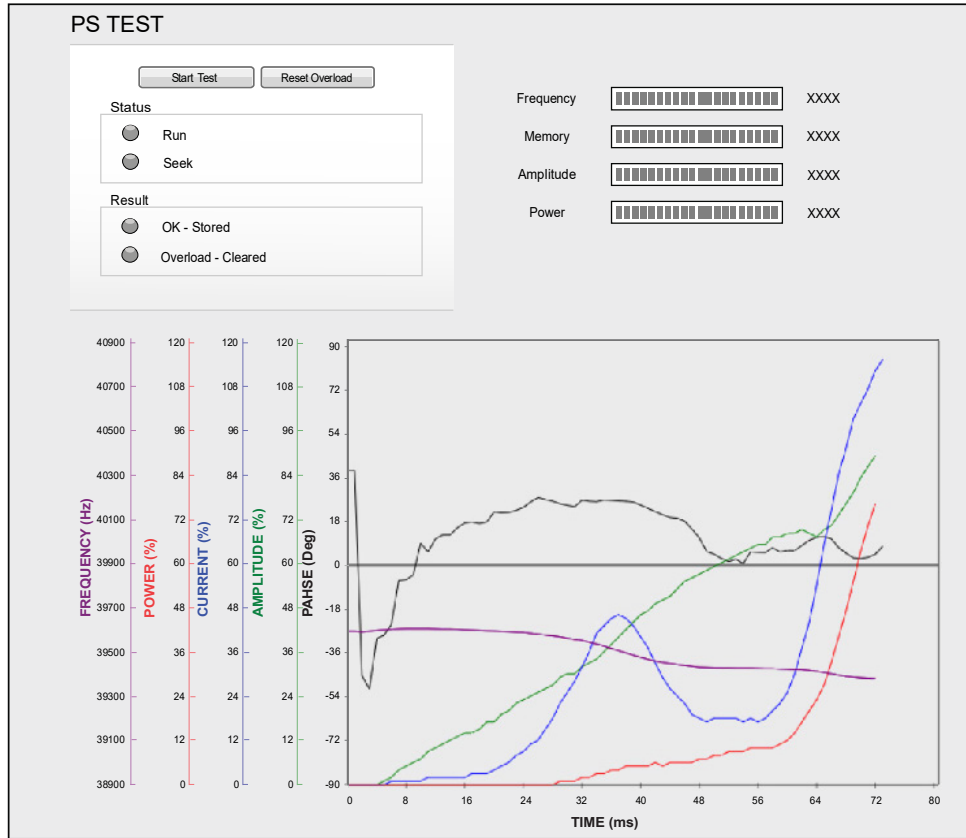
Figure A.10 Weld Graph, Defective Horn
