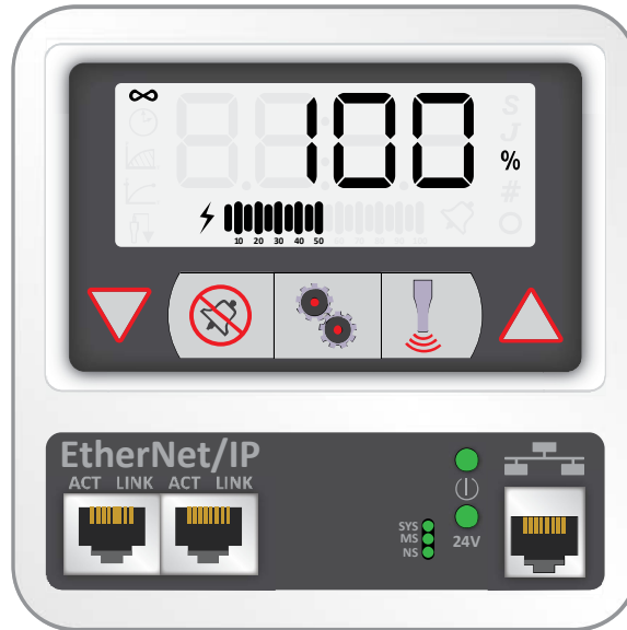
Figure 2.3 DCX F-EIP Power Supply Front Panel Controls and Indicators
