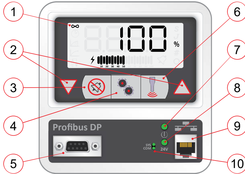
Figure 2.3 DCX Power Supply F-DP Front Panel Controls and Indicators
