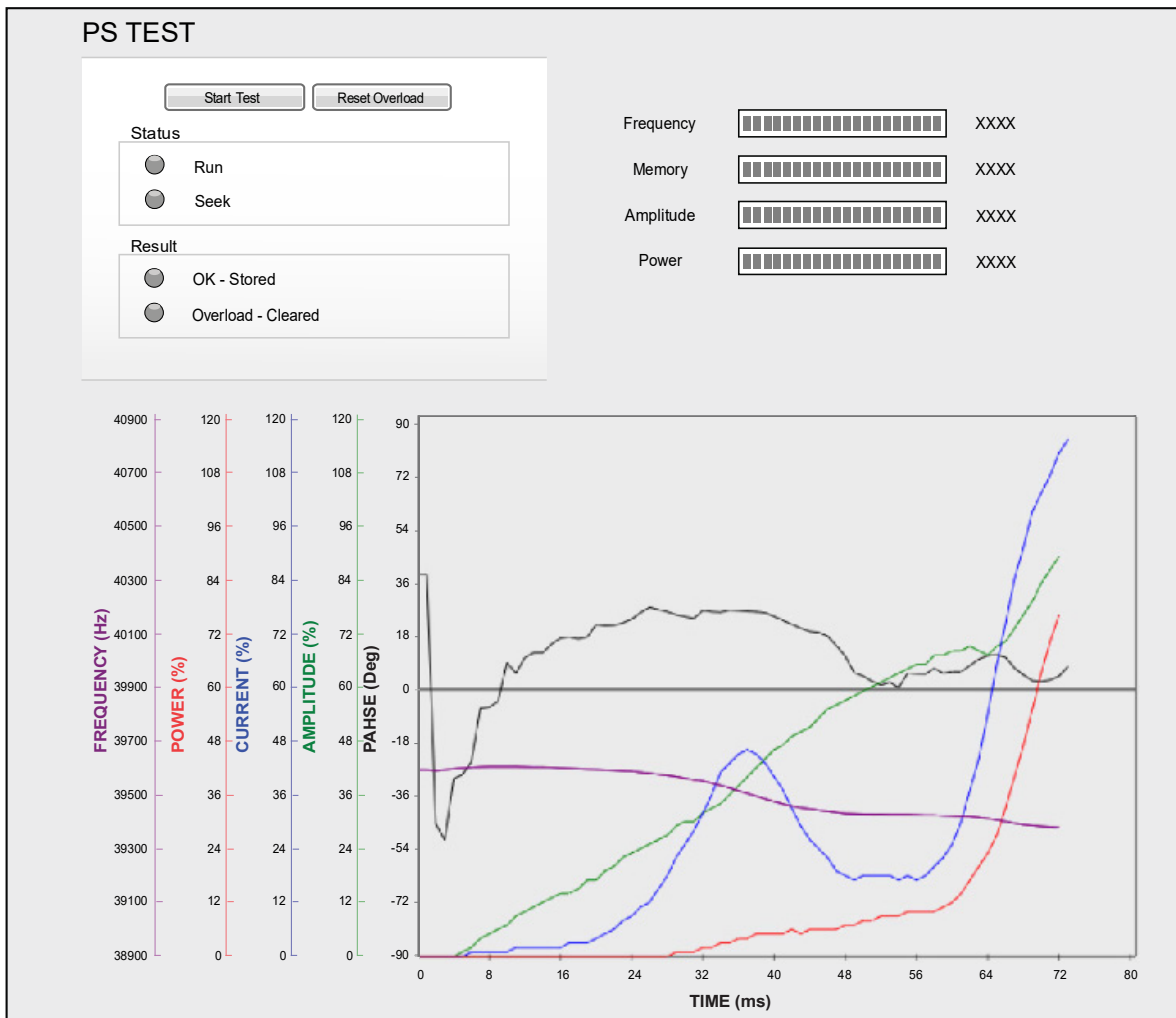
Figure A.10 Weld Graph, Defective Horn
