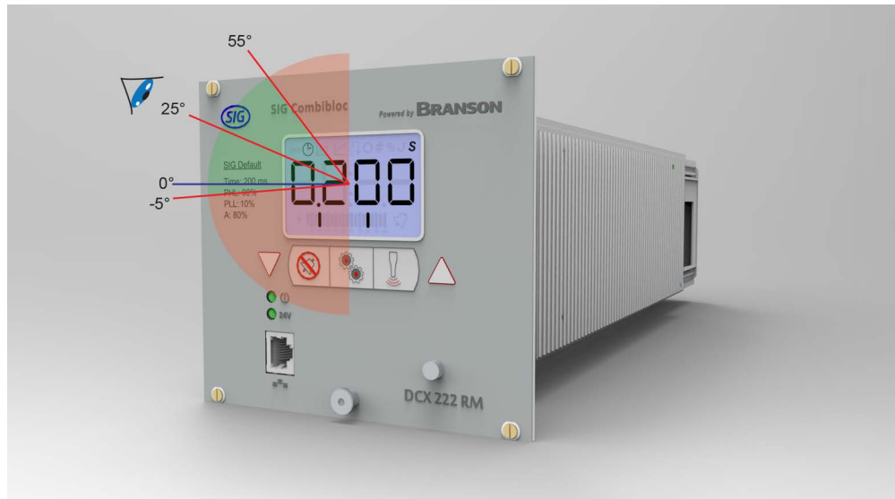
Figure 5.2 LCD Viewing Angle
