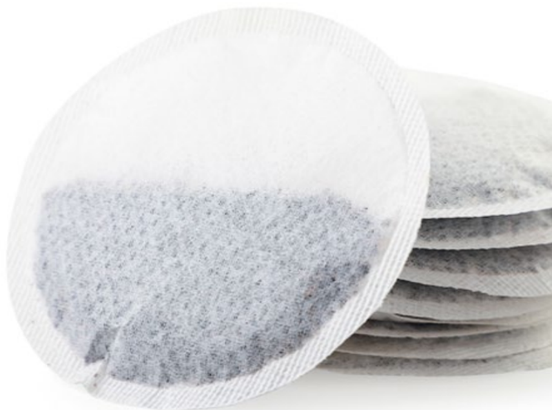
New, single-use teabag designs place leaf tea between two discs of porous, nonwoven PLA (polylactic acid) mesh that are ultrasonically plunge-welded together. PLA is an industrially compostable BDCP.
