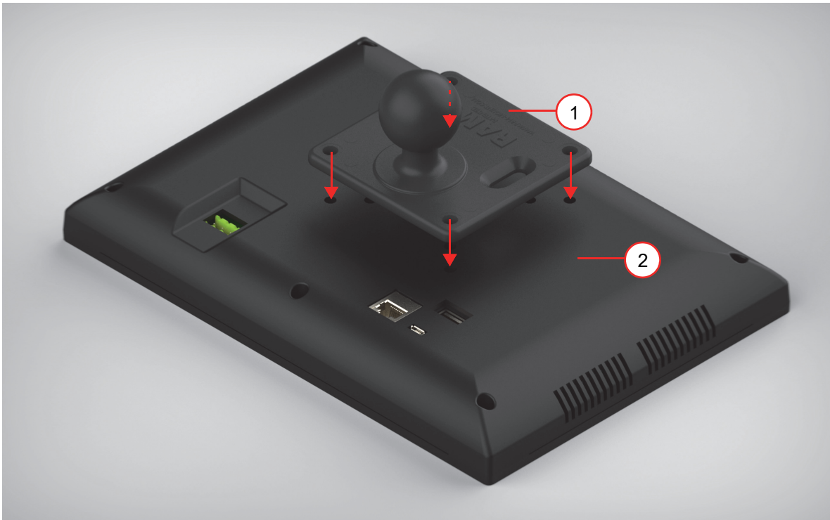
Figure 4.6 Attaching HMI to Mounting Plate
