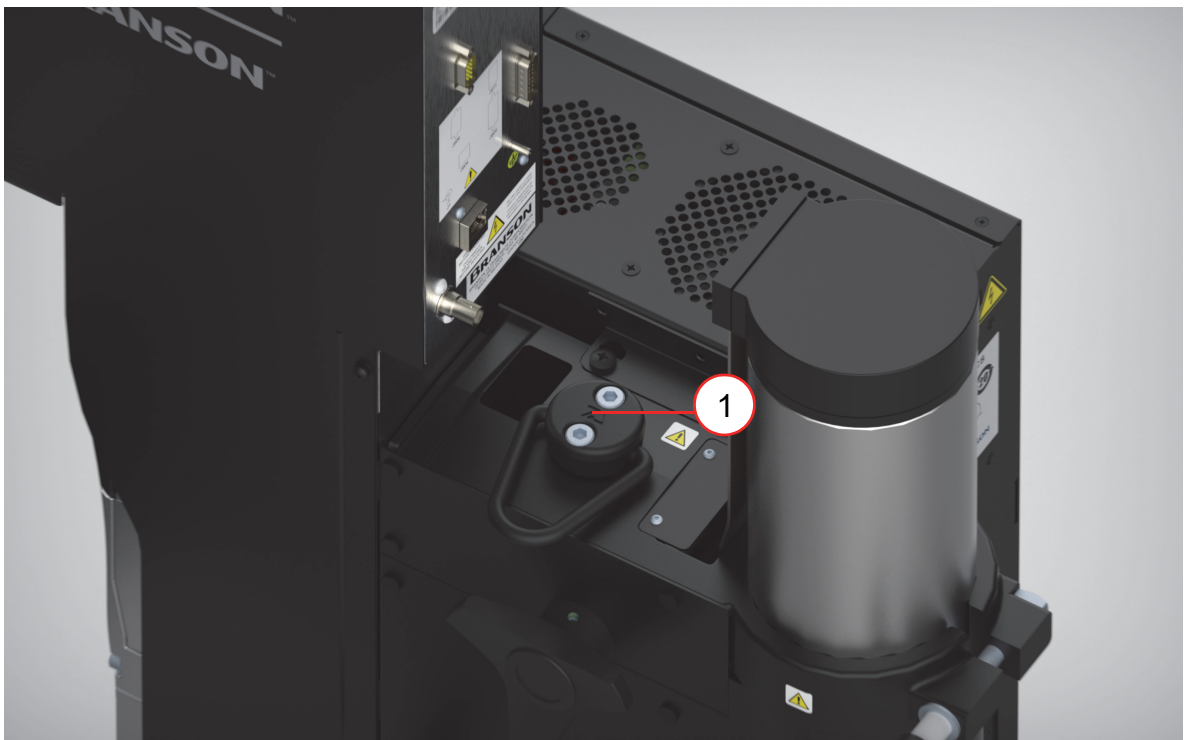
Figure 4.1 Lift Point Location - Round Column
