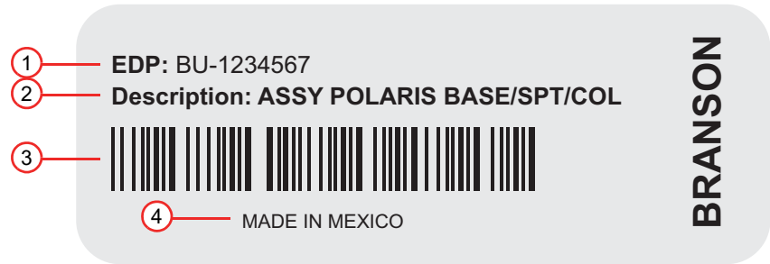
Figure 2.11 System Information Label - Base
