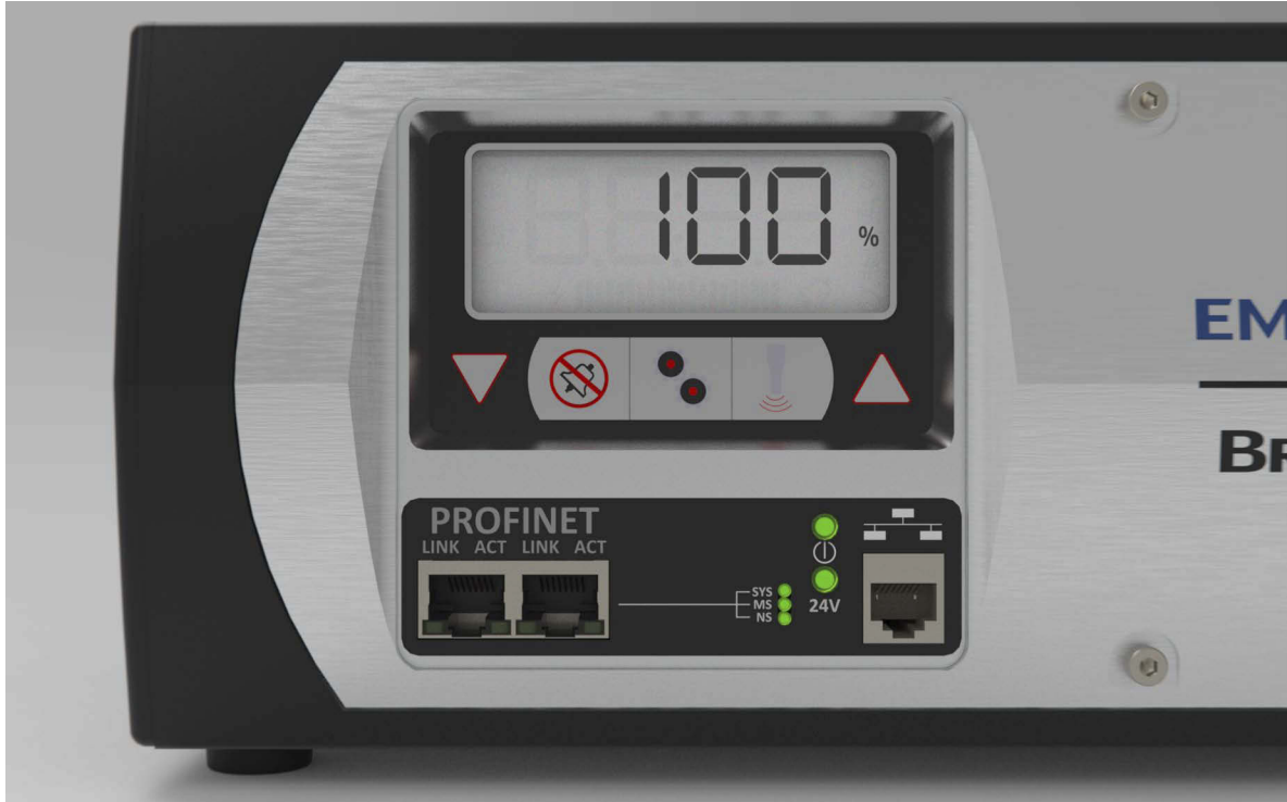
Figure 2.8 DCX F-PFN Power Supply Front Panel Controls and Indicators
