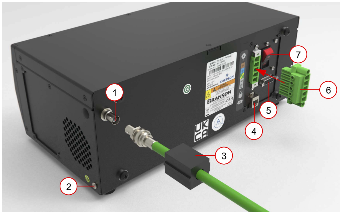
Figure 5.2 DCX F-PFN Power Supply Connections - Horizontal
