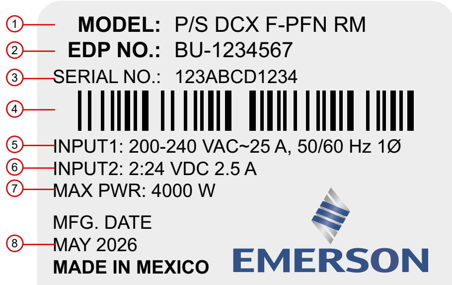
Figure 1.1 System Information Label - Power Supply
