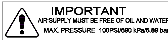
Figure 1.3 Caution label on the 2000X aed Actuator for the factory air supply
