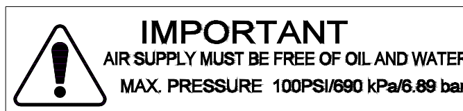
Figure 1.2 Caution label on the aod Actuator for the factory air supply
