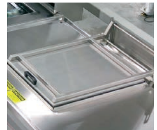
Dry – Typically, drying is accomplished via re-circulated hot air with optional HEPA filtration.
